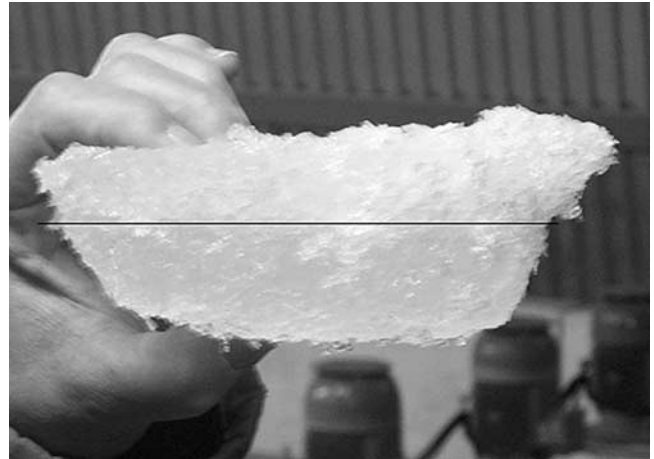
Figure 3. Photograph of a type C pancake grown in the HSVA ice tank. The horizontal line divides the more open, porous, top layer from the more consolidated lower layer.
